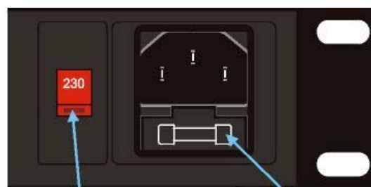
Voltage Selector Fuses under flap
